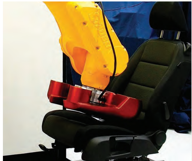
ATI F/T Sensor used in automotive seat testing.
