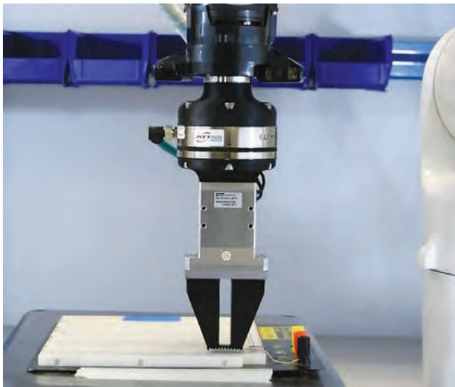
ATI F/T Sensor utilized in precision electronic assembly.
